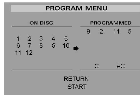
The left hand of the screen will display all available chapters (songs) on the current disc up to a maximum of 30. Scroll through these using the ◀ or ▶ keys and press the **ENTER** key once you have selected a desired song. The number of the selected song should then appear on the right side of the same screen. Repeat the process for a maximum of 30 choices.
